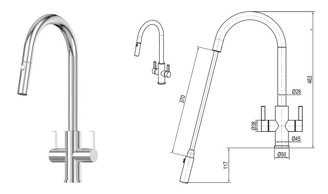
Note: Drawings are not to scale and are for reference only. Specifications and sizes can be changed by the manufacturer without notice. Refer to physical unit prior to installation.
