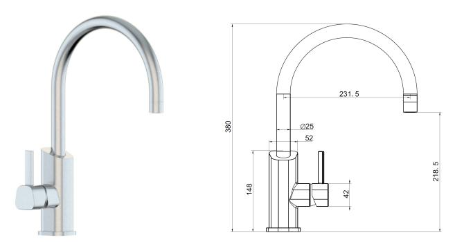
Note: Drawings are not to scale and are for reference only. Specifications and sizes can be changed by the manufacturer without notice. Refer to physical unit prior to installation.
