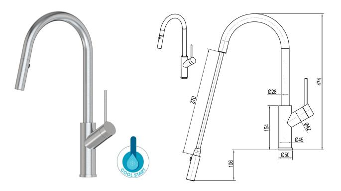
Note: Drawings are not to scale and are for reference only. Specifications and sizes can be changed by the manufacturer without notice. Refer to physical unit prior to installation.
